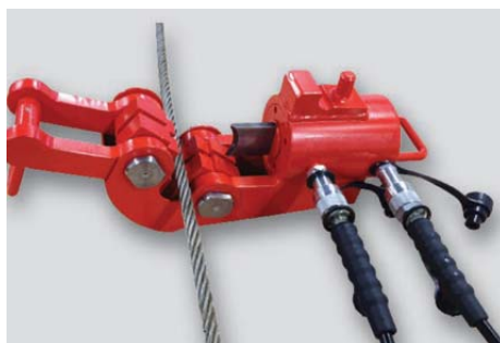
Step 2: Position material to be cut in the cutting head slot.
